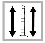
8. During the reaction period, close the mixing cylinder and vigorously shake the prepared sample. The sample becomes reddish-orange, brown or blue. The color is dependent on the zinc concentration.
