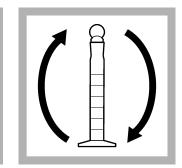
**4.** Close the cylinder. Invert the cylinder several times to dissolve the powder completely. Inconsistent readings may result if all the particles are not dissolved.
