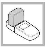
**18.** Install the instrument cap over the cell holder.
