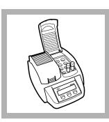
**3.** Insert the reaction tube in the preheated DRB200 reactor. Close the lid.
