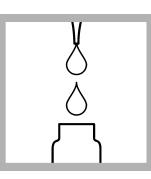
**10.** Use a pipet to slowly add 1.0 mL of undigested sample to a test vial 2 (green label).
