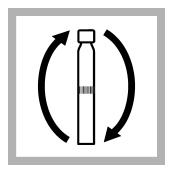
**9.** Quickly tighten the cap on the vial and invert until completely mixed. Immediately continue to the next step.
