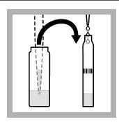
**7.** Use a pipet to slowly add 0.5 mL of the digested sample from the 20-mm reaction tube into a test vial 1 (red label).
