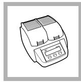
1. Set the DRB200 reactor power to on. Set the temperature to 120 °C (248 °F).
