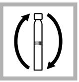
**12.** Quickly tighten the cap on the vial and invert until completely mixed.
