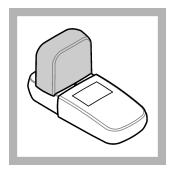
**13.** Install the instrument cap over the cell holder.
