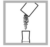
**4.** Add the contents of one Molybdenum 1 Reagent Powder Pillow to the mixing cylinder.
