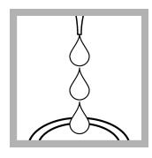
7. Develop the sample: Add 0.5 mL of Molybdenum 2 Reagent Solution to the prepared sample cell.
