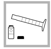
**10. Prepare the blank:** When the timer expires, fill a second sample cell with 10 mL of the prepared sample.
