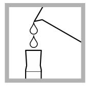
**2. Prepare the sample:** Fill a 25-mL graduated mixing cylinder with 5 mL of sample.
