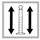
**5.** Close the cylinder. Gently shake or invert the cylinder to completely dissolve the reagent.
