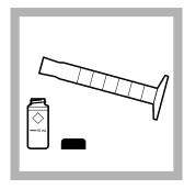
**6.** Fill a sample cell with 10 mL of the prepared sample.
