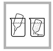
3. Prepare the blank: Pour at least 40 mL of deionized water into a 50-mL beaker. Fill an AccuVac Ampul with deionized water. Keep the tip immersed while the AccuVac Ampul fills completely.
