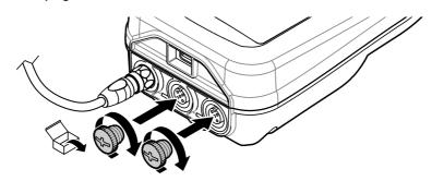
Figure 7 USB port plug installation
