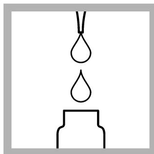
7. Add 2 mL of 1.00 N Sodium Hydroxide to the vial. Cap the vial and shake to mix.
