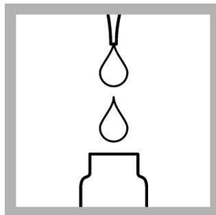
3. Add 5.0 mL of sample to the Total and Acid Hydrolyzable Test Vial. Close the vial and mix.
