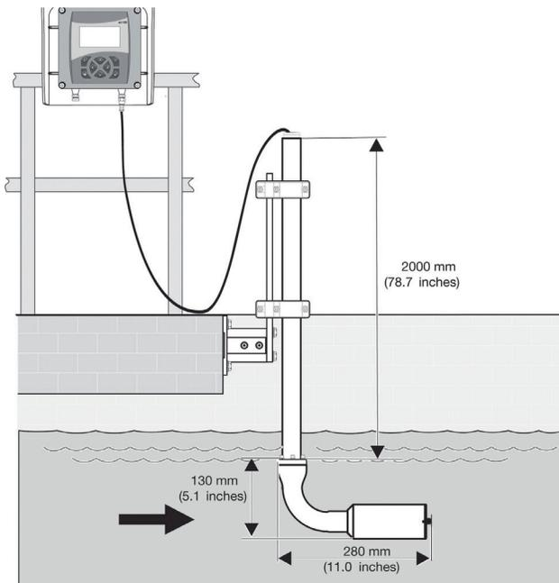
*Fixture with ball valve for mounting Solitax sc models
