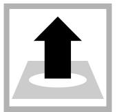
**10.** Remove the blank AccuVac Ampul from the cell holder.
