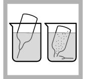
2. Prepare the blank: Pour at least 40 mL of deionized water in a 50-mL beaker. Fill one SPADNS or SPADNS2 Fluoride Reagent AccuVac Ampul with deionized water. Keep the tip immersed while the Ampul fills completely.
