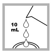
5. Prepare the sample: Fill a second sample cell with 10 mL of sample.
