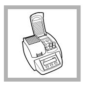
**7.** Insert the vials in the preheated DRB200 Reactor. Close the cover.
