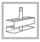
**9.** After the timer expires, let the vials cool in a test tube rack for 2 minutes. If the solution develops a colorless upper layer and a purple lower layer, invert the vials several times to mix. Use finger cots to touch hot vials.
