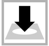
**14.** Insert the blank vial into the 16-mm cell holder.
