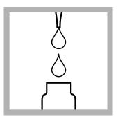
**4. Prepare the sample:** Use a pipet to add 0.5 mL of the homogenized sample to a test vial.
