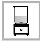
**3.** Add a stir bar and put the beaker on a magnetic stirrer. Stir at a moderate rate.
