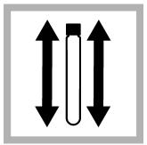
**3.** Put the cap on the vial. Shake to dissolve the powder. A pink color shows if nitrite-nitrogen is present in the sample.
