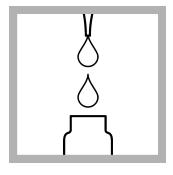
**5. Prepare the blank:** When the timer expires, fill an empty Test 'N Tube vial with 5 mL of sample.
