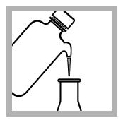
**5.** If the sample volume is less than 50 mL, dilute to approximately 50 mL with deionized water.
