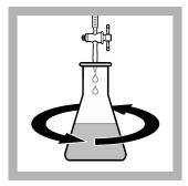
**10.** Put the flask under the buret. Swirl the flask. Add titrant until the color changes from red to pure blue.
