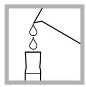
**3.** Use a graduated cylinder or pipet<sup>1</sup> to measure the sample volume from Table 1 on page 3.
