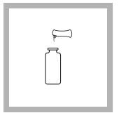
**4.** Add the contents of one SulfaVer 4 Reagent Powder Pillow to the sample cell (the prepared sample). Swirl to mix.
