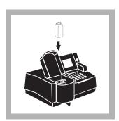
**9.** Within five minutes after the timer beeps, place the prepared sample into the cell holder. Close the light shield. Results in mg/L sulfate (or chosen units) will be displayed.
