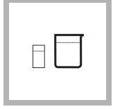
**4.** Fill a Zeroing Vial with at least 10 mL of sample (the blank). Collect at least 40 mL of sample in a 50-mL beaker.
