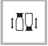
**6.** Quickly invert the ampul several times to mix. Wipe off any liquid or fingerprints.
