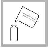
**3.** Fill a clean sample cell with 25 mL of sample.
