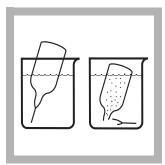
**5.** Fill a SulfaVer 4 Sulfate AccuVac Ampul with sample (the prepared sample).
