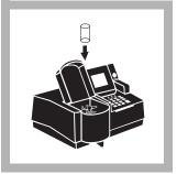
**8.** When the timer beeps, place the blank in the cell holder. Close the light shield.
