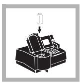
**7.** When the timer beeps, place the blank in the cell holder. Close the light shield.
