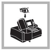
**3.** Insert the 1-inch Cell Adapter into the sample cell module by sliding it under the thumb screw and into the alignment grooves. Fasten with the thumb screw.
