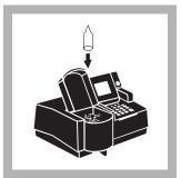
10. Within five minutes after the timer beeps, place the prepared sample into the cell holder. Close the light shield. Results in mg/L sulfate (or chosen units) will be displayed.
