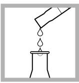
2. Add 10 mL of sample to a 50-mL Erlenmeyer flask. Put the stir bar in the Erlenmeyer flask.
