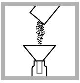
5. Add the contents of one **TOC Persulfate Powder** Pillow to each Acid Digestion Vial. Put a label that says "Reagent Blank" on one Mid Range Acid Digestion vial. Put a lable that says "Sample" on a second Mid Range Acid Digestion vial.
