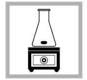
**4.** Put the flask on a stir plate. Stir at a moderate speed for 10 minutes.
