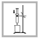
7. Soak the cotton plug with deionized water and compress it with the plunger. Remove the plunger. If the cotton plug moves up the column, push it back to the bottom with a clean, blunt rod.
