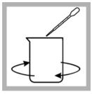
3. Using a plastic 1mL dropper, add 1.0 mL of pPb-1 Acid Preservative Solution to the sample and swirl to mix.
