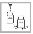
**18.** Remove the sample cell and add 3 drops of pPb-6 Decolorizer Solution to the cell. Swirl vigorously to mix
