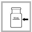
14. Pour 10 mL of solution into a sample cell.
