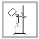
8. Pour the prepared sample slowly into the center of the Column Extractor. Wait for the sample to flow through.
