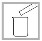
2. Fill a 100 mL plastic graduated cylinder with 100 mL of the sample. Pour the measured sample into a 250 mL plastic beaker.
