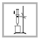
After the flow has stopped, fully compress the absorbent pad in the Extractor with the plunger. Discard the contents of the beaker. Slowly withdraw the plunger from the Extractor.
