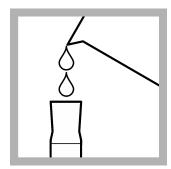
3. Use a graduated cylinder or a pipet<sup>1</sup> to measure the sample volume from Table 1 on page 3.
