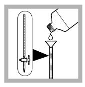
**2.** Fill a 25-mL buret to the zero mark with the titrant.
