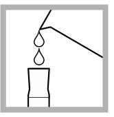
**4.** Use a graduated cylinder or a pipet<sup>1</sup> to measure the sample volume from Table 1 on page 4.
