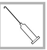
2. Insert a clean delivery tube into the digital titration cartridge. Attach the cartridge to the Digital Titrator.
