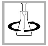
**11.** Put the end of the delivery tube fully into the solution. Swirl the flask. Turn the knob on the Digital Titrator to add titrant to the solution. Continue to swirl the flask. Add titrant until the color changes from red to pure blue. Record the number of digits on the counter.
