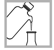
**8.** If the sample volume is less than 100 mL, dilute to approximately 100 mL with deionized water.
