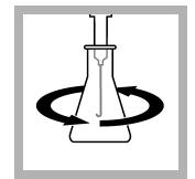
**11.** Put the end of the delivery tube fully into the solution. Swirl the flask. Turn the knob on the Digital Titrator to add titrant to the solution. Continue to swirl the flask. Add titrant until the color changes from red to pure blue. Record the number of digits on the counter.
