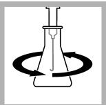
**10.** Put the end of the delivery tube fully into the solution. Swirl the flask. Turn the knob on the Digital Titrator to add titrant to the solution. Continue to swirl the flask. Add titrant until the color changes to pale yellow.
