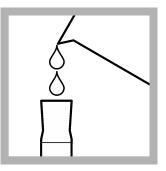
**4.** Use a graduated cylinder or a pipet<sup>1</sup> to measure the sample volume from Table 1 on page 3.
