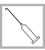
2. Insert a clean delivery tube into the digital titration cartridge. Attach the cartridge to the Digital Titrator.
