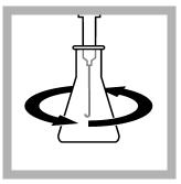
**10.** Put the end of the delivery tube fully into the solution. Swirl the flask. Turn the knob on the Digital Titrator to add titrant to the solution. Continue to swirl the flask. Add titrant until the color changes to light pink. Record the number of digits on the counter.
