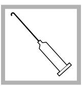
**3.** Insert a clean delivery tube into the digital titration cartridge. Attach the cartridge to the Digital Titrator.
