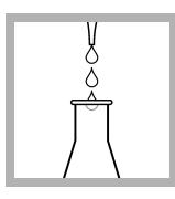
**7.** Add 5 drops of 5.25 N Sulfuric Acid Standard Solution.
