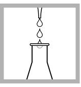
6. If the sample volume is 100 mL, add 2 mL of 8 N Potassium Hydroxide Standard Solution. If the sample volume is 50 mL or less, add 1 mL of 8 N Potassium Hydroxide Standard Solution.
