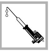
2. Hold the Digital Titrator with the cartridge tip up. Turn the delivery knob to eject air and a few drops of titrant. Reset the counter to zero and clean the tip.
