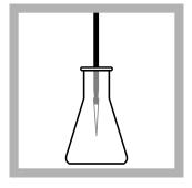
8. Use a TenSette pipet with a new tip to add 0.2 mL of bleach sample to the flask. Make sure to add the sample below the solution level.
