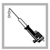
4. Hold the Digital Titrator with the cartridge tip up. Turn the delivery knob to eject air and a few drops of titrant. Reset the counter to zero and clean the tip.
