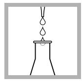
**13.** Add 1 mL of 5.25 Sulfuric Acid Standard Solution.
