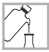
**6.** If the sample volume is less than 50 mL, dilute to approximately 50 mL with deionized water.
