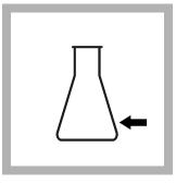
**3.** Fill a clean 125-mL Erlenmeyer flask to approximately the 75-mL mark with deionized water or tap water.
