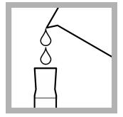
5. Use a graduated cylinder or a pipet to measure the sample volume from Table 1 on page 3.
