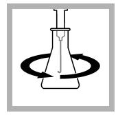
**11.** Put the end of the delivery tube fully into the solution. Swirl the flask. Turn the knob on the Digital Titrator to add titrant to the solution. Continue to swirl the flask. Add titrant until the color changes from orange to pale blue. Record the number of digits on the counter.
