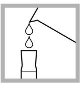
**4.** Use a graduated cylinder or a pipet<sup>1</sup> to measure the sample volume from Table 1 on page 3.
