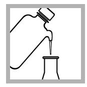
7. If the sample volume is less than 150 mL, dilute to approximately 150 mL with deionized water.
