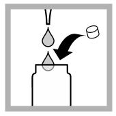
2.0 mL of Solution A and 1 Reagent B tablet in quick succession to a dry 20-mm reaction tube. Close the reaction tube
