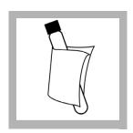
11. Clean the outer surface of the vial with a damp cloth. Dry the vial with a dry cloth to remove fingerprints and other marks.
