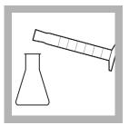
4. Use a 100-mL graduated cylinder to measure 75 mL of concentrated sulfuric acid. Add the acid to a 250 mL plastic Erlenmeyer flask.
