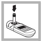
**12.** After the timer beeps, put the **blank** into the adapter. Push straight down on the top of the vial until it is fully installed. The vial must not move, because this can cause reading errors.
