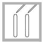
7. Add 0.2 mL of sample to one vial (the sample) and 0.2 mL of deionized water to the other vial (the blank).
