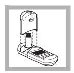
**15.** Put the prepared **sample** in the adapter. Put the instrument cap over the vial. Push straight down on the top of the vial until it is fully installed. The vial must not move, because this can cause reading errors.
