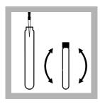
**9.** Add 3.5 mL of the BoroVer 3 solution prepared in step 5 to the blank vial. Tighten the cap and invert to mix.
