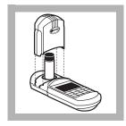
**13.** Put the instrument cap over the vial.
