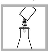
7. Add the contents of one Phenolphthalein Indicator Powder Pillow. The indicator is not necessary if a pH meter is used.
