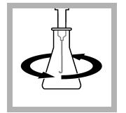
**9.** Put the end of the delivery tube fully into the solution. Swirl the flask. Turn the knob on the Digital Titrator to add titrant to the solution. Continue to swirl the flask. Add titrant until the color changes from pink to colorless, or until the pH is 8.3. Record the number of digits on the counter.
