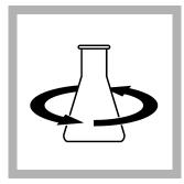
**8.** Swirl to mix. If the solution is colorless or the pH is less than 8.3, the Phenolphthalein alkalinity is zero. Go to step **11**.
