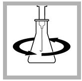
**13.** Put the end of the delivery tube fully into the solution. Swirl the flask. Turn the knob on the Digital Titrator to add titrant to the solution. Continue to swirl the flask. Add titrant until the color changes to a light pink color, or the pH is 4.5 (refer to Table 2 on page 3 for additional pH endpoints). Record the number of digits on the counter.
