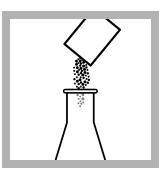
**11.** Add the contents of one Bromcresol Green-Methyl Red Indicator Powder Pillow. The indicator is not necessary if a pH meter is used.
