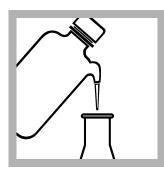
**6.** If the sample volume is less than 100 mL, dilute to approximately 100 mL with deionized water.
