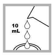
**20.** Prepare the blank: Put at least 10 mL of chloroform in a dry sample cell. Put the stopper on the sample cell.
