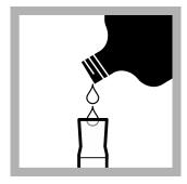
**6. Prepare the DithiVer solution:** Add 30 mL of chloroform to a 50-mL mixing cylinder.
