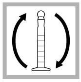
**8.** Put the stopper on the mixing cylinder. Invert the mixing cylinder several times to mix.
