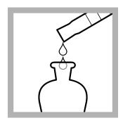
**9.** Add 20 mL of 50% Sodium Hydroxide Solution to the funnel.
