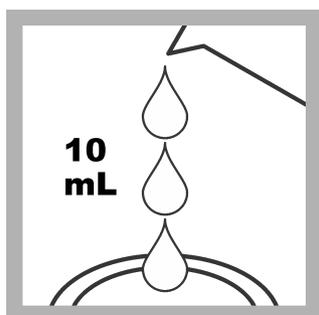
6. **Prepare the sample:** Fill a second sample cell with 10 mL of sample. Mix the sample well before it is added to the sample cell.
