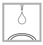
9. Prepare the blank: Add 1 drop of ECR Masking Reagent Solution into a second clean sample cell.
