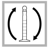
mixing cylinder. Invert the mixing cylinder several times to fully dissolve the powder.
