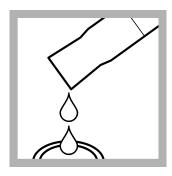
**10.** Pour 10 mL of the remaining solution from the mixing cylinder into the blank sample cell.
