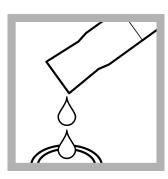
**8.** Pour 10 mL of the solution from the mixing cylinder into a clean sample cell.
