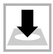
**17.** Within 5 minutes after the timer expires, insert the prepared sample into the cell holder.
