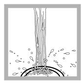
4. Rinse a clean plastic sample cell and the cap three times with the sample. Do not let the interior surface of the cap touch surfaces that can have contamination.
