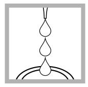
**6.** Use a pipet to add 0.5 mL of Molybdate 3 Reagent solution to the sample cell.
