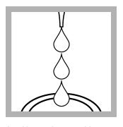
**15.** Use a pipet to add 0.5 mL of Amino Acid F Reagent solution to the sample cell.
