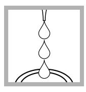
**9.** After the timer expires, use a pipet to add 0.5 mL of Citric Acid F Reagent solution to the sample cell.
