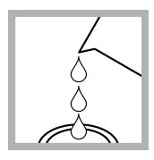
**5.** Fill the sample cell to the 25-mL mark with sample.
