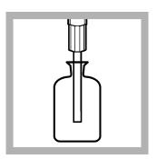
**4.** Remove the stopper. Put the probe in the bottle.
