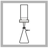
3. Assemble the 0.45 micron filter apparatus. **NCASI:** The NCASI test uses a 0.8-micron filter. A 1.0 micron prefilter can be used first for samples that are difficult to filter.
