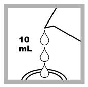
**8. Prepare the sample:** Fill a second sample cell with 10 mL of filtered sample.
