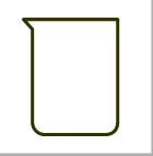
2. Collect 200 mL of sample in a 400-mL beaker. NCASI: Adjust the pH as described in Before starting on page 1.
