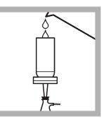
**4.** Pour approximately 50 mL of deionized water through the filter to rinse the filter. Discard the rinse water.
