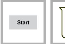
1. Start program 120 Color, 455 nm or program 125 Color, 465 nm for the NCASI test. Colorimeters use program 122 Color, 420 nm. For information about sample cells, adapters or light shields, refer to Instrument-specific information on page 1.
