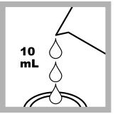
6. Prepare the blank: Fill the sample cell with 10 mL of filtered deionized water from the previous step. Discard the excess water in the flask.
