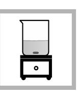
**3.** Add a stir bar and put the beaker on a magnetic stirrer. Stir at a moderate rate.
