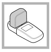
**11.** Install the instrument cap over the cell holder.
