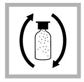
**4.** Quickly invert the AccuVac Ampuls several times to mix. Some of the blue color will be bleached if ozone is in the sample.
