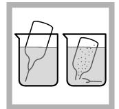
2. Prepare the blank: Pour at least 40 mL of ozone-free water in a 50-mL beaker. Fill an Indigo Ozone Reagent AccuVac Ampul with the ozone-free water. Keep the tip immersed while the Ampul fills fully, then immediately put the stopper on the tip.
