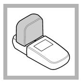
**7.** Install the instrument cap over the cell holder.
