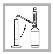
**5.** Use the bottle-top dispenser to add 1.0 mL of prepared Total Chlorine Indicator Solution to the same mixing cylinder.
