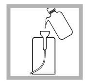
**12.** Flush the Pour-Thru Cell with at least 50-mL of deionized water immediately after use.
