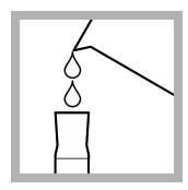
**7.** Carefully fill the same mixing cylinder to the 80-mL mark with sample.
