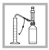
**4.** Use the bottle-top dispenser to add 1.0 mL of Total Chlorine Buffer Solution to a clean, dry 100-mL glass mixing cylinder.
