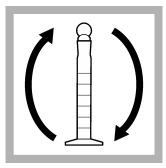
**8.** Put the stopper on the mixing cylinder. Invert the mixing cylinder carefully several times to mix. Continue to the next step immediately.
