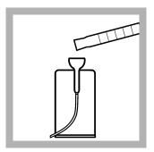
10. When the timer expires, fill the funnel of the Pour-Thru Cell with the reacted sample from the mixing cylinder. It is not necessary to pour all of the sample into the Pour-Thru Cell; discard approximately half of the sample.
