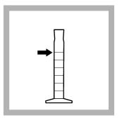
**3.** Fill the rinsed cylinder to the 25-mL mark with sample.
