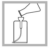
**12.** When the timer expires, pour the contents of the Erlenmeyer flask that contains the blank into the Pour-Thru Cell.
