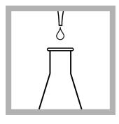
9. Prepare the sample: Use the micropipette to add 1.0 mL of prepared Ascorbic Acid reagent to one of the Erlenmeyer flasks. The remaining Erlenmeyer flask is the blank.
