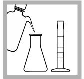
2. Rinse two clean Erlenmeyer flasks and one clean graduated cylinder three times with the sample.
