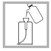
**16.** Flush the Pour-Thru Cell with at least 50-mL of deionized water immediately after use.
