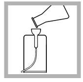
**14.** Pour the contents of the Erlenmeyer flask that contains the prepared sample into the Pour-Thru Cell.
