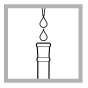
**1.** Use a pipet to add 5 mL of Nitrate ISA solution into a 100-mL volumetric flask.
