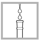
1. Use a pipet to add 5 mL of Nitrate ISA Solution into a plastic 100-mL volumetric flask.
