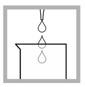
**8.** Add 0.4 mL of 10-mg/L Nitrate Nitrogen Standard Solution to make a 0.04-mg/L standard solution.
