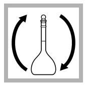
**3.** Insert the stopper. Invert the flask to mix.
