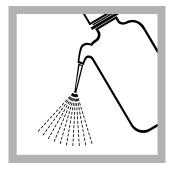
**12.** Rinse the probe with deionized water. Dry the probe with a lint-free cloth.
