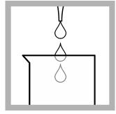
**14.** Add 1.2 mL or 2.0 mL of 100-mg/L Nitrate Nitrogen Standard Solution to make a 1.2-mg/L or 2.0-mg/L standard solution.
