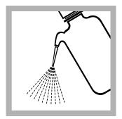
**10.** Rinse the probe with deionized water. Dry the probe with a lint-free cloth.
