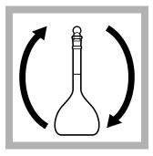
**3.** Insert the stopper. Invert the flask to mix.
