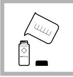
2. Prepare the sample: Rinse a sample cell and cap three times with sample. Fill the sample cell to the 10-mL mark with sample.
