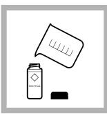
6. Prepare the blank: Rinse a sample cell and cap three times with sample. Fill the sample cell to the 10-mL mark with sample. Close the sample cell.
