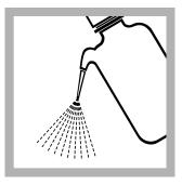
**4.** Rinse the probe with deionized water. Dry the probe with a lint-free cloth.
