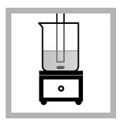
**5.** Put the probe in the solution. Do not let the probe touch the stir bar, bottom or sides of the container. Remove the air bubbles from under the probe tip.
