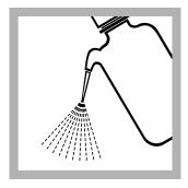
**8.** Rinse the probe with deionized water. Dry the probe with a lint-free cloth.
