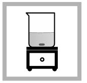
**3.** Add a stir bar and put the beaker on a magnetic stirrer. Stir at a moderate rate.
