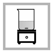
**3.** Add a stir bar and put the beaker on a magnetic stirrer. Stir at a moderate rate.
