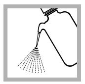
**7.** Rinse the probe with deionized water. Dry the probe with a lint-free cloth.
