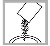
**9.** Add one 10-mL DPD Free Chlorine Reagent Powder Pillow or one 10-mL DPD Total Chlorine Reagent Powder Pillow to the second sample cell.
