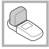
**5.** Install the instrument cap over the cell holder.
