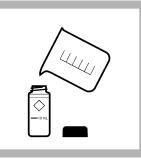
2. Prepare the blank: Rinse a sample cell and cap three times with sample. Fill the sample cell to the 10-mL mark with sample. Close the sample cell.
