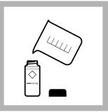
8. Prepare the sample: Rinse a second sample cell and cap three times with sample. Fill the sample cell to the 10-mL mark with sample.
