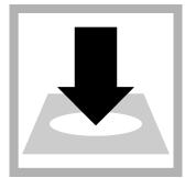
**14. Total chlorine measurement:** Within 6 minutes of the reagent addition, insert the prepared sample AccuVac Ampul into the cell holder.
