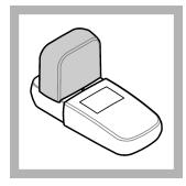
**15.** Install the instrument cap over the cell holder.
