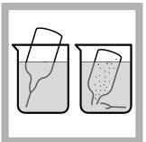
8. Prepare the sample: Collect at least 40 mL of sample in a 50-mL beaker. Fill a DPD Free Chlorine Reagent AccuVac Ampul or a DPD Total Chlorine Reagent AccuVac Ampul with sample. Keep the tip immersed while the AccuVac Ampul fills completely.
