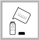
2. Prepare the blank: Rinse a sample cell and cap three times with sample. Fill the sample cell to the 10-mL mark with sample. Close the sample cell.
