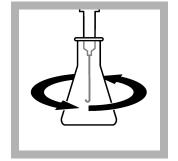
7. Put the end of the delivery tube fully into the solution. Swirl the flask. Turn the knob on the Digital Titrator to add titrant to the solution. Continue to swirl the flask. Add titrant until the color changes from colorless to a light pink color for a minimum of 30 seconds (pH 8.3). Record the number of digits on the counter.
