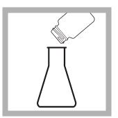
**4.** Pour the sample volume in Table 1 on page 2 in a 250-mL Erlenmeyer flask. When possible, collect the sample directly in the Erlenmeyer flask to prevent agitation of the sample.
