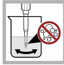
3. Shake the probe from side to side to refresh the reference junction and remove air bubbles.
