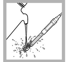
4. Rinse the probe with deionized water. Dry the probe with a lint-free cloth.
