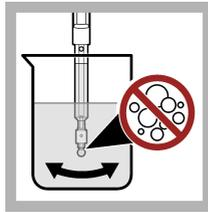
6. Shake the probe from side to side to refresh the reference junction and remove air bubbles.
